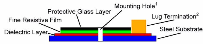
A heat sink can be mounted to the resistor to increase size to power dissipation ratio.
